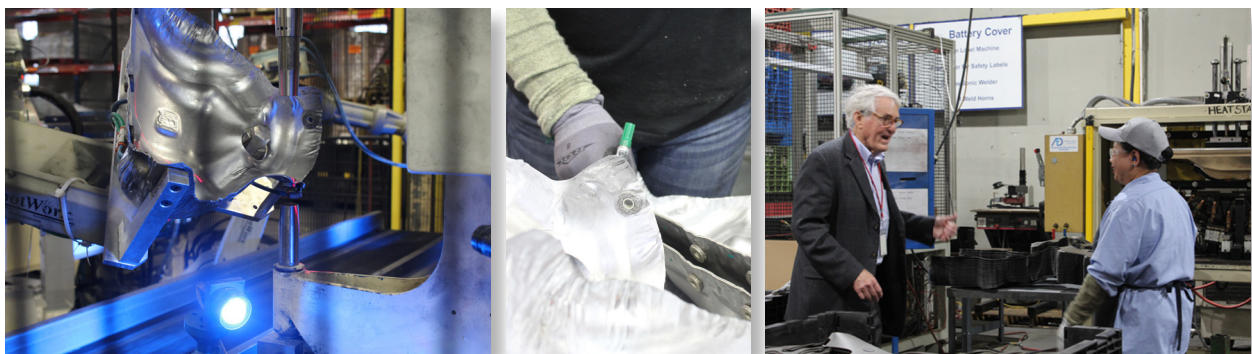
(Photos from left to right) At Cleveland-based manufacturer Soundwich, the blue light of this robotic system reflects off of parts and identifies whether they are correctly made. After a 360-degree review, robotic arms place correct parts on one conveyer belt and faulty ones on another. • This worker at Soundwich in Cleveland uses a green marker to place “witness marks,” which indicate to customers that people have checked the quality of the parts being manufactured. • Dan T. Moore, whose namesake company owns 10 manufacturing companies, speaks with Vannak So, who’s worked for one company, Soundwich, for more than 30 years.
